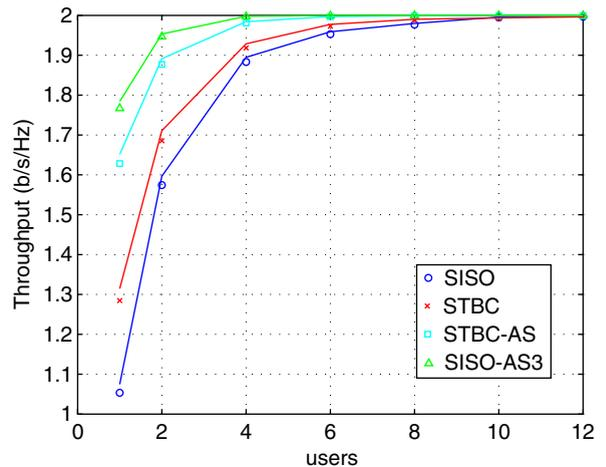
Fig. 4. Link throughput vs. the number of users for the different transmission schemes in an unlimited feedback scenario ( $\bar{\gamma} = 10$  dB,  $L = 50$ ). Solid line: simulation, symbols: analytical expression.
