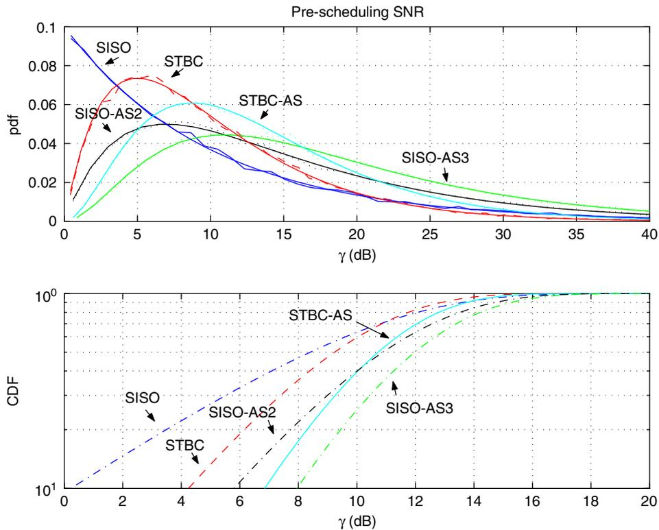
Fig. 1. Top: Analytical and simulated curves for the probability density functions of the pre-scheduling SNRs. Bottom: Cumulative density functions in log-scale. ( $\bar{\gamma} = 10$  dB).
