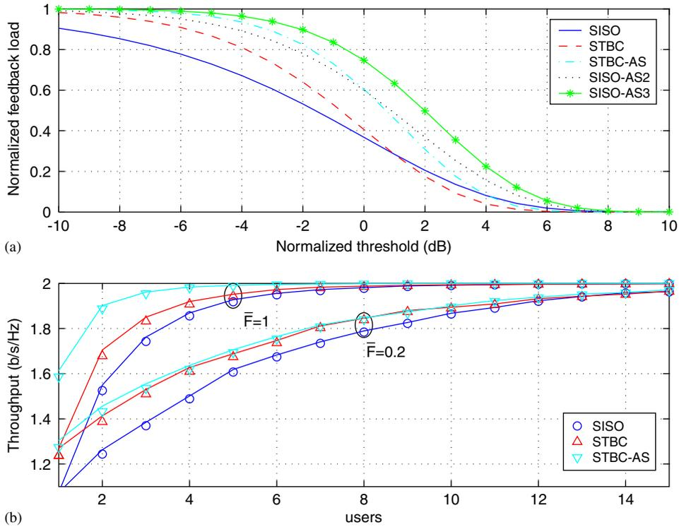
Fig. 6. (a) Normalized feedback load vs. normalized threshold  $\gamma_{th}/\bar{\gamma}$  for the different transmission schemes. (b) Analytical (symbols) vs. simulation (solid) results for the different transmission schemes.
