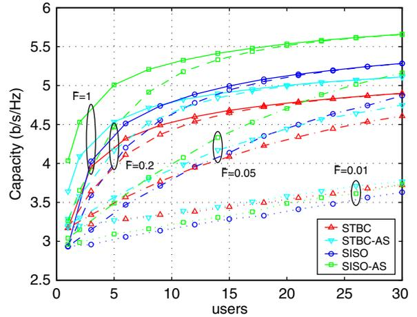
Fig. 7. Channel capacity vs. number of users for the different transmission schemes and feedback loads  $\bar{F} = 1$  (solid), 0.2 (dashed), 0.05 (dash-dotted), 0.01 (dotted).  $\bar{\gamma} = 10$  dB.
