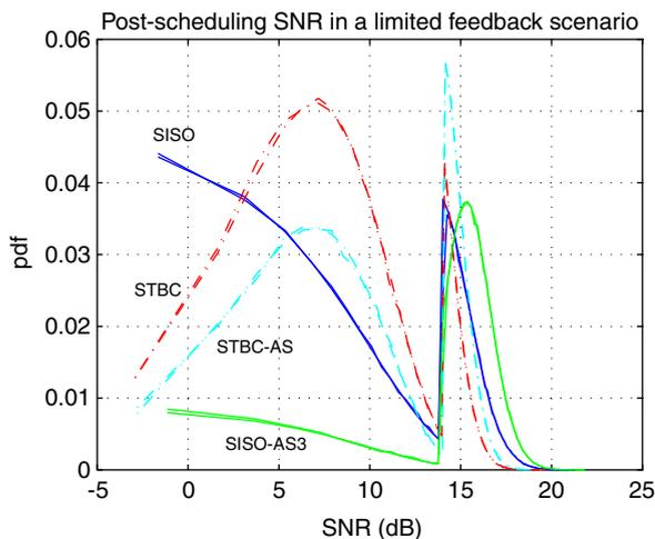
Fig. 5. Analytical and simulated pdf of the post-scheduling SNR for the different transmission schemes in a limited feedback scenario ( $\bar{\gamma} = 10$  dB,  $\gamma_{\text{th}} = 14$  dB, 10 users).
