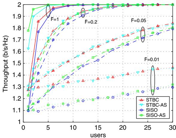
Fig. 8. Link layer throughput vs. number of users for the different transmission schemes and feedback loads  $\bar{F} = 1$  (solid), 0.2 (dashed), 0.05 (dash-dotted), 0.01 (dotted).  $\bar{\gamma} = 10$  dB. QPSK.
