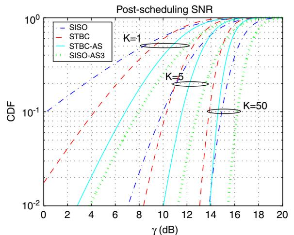
Fig. 2. CDF of the received SNR for the different transmission schemes, for  $K = 1, 5, 50$  users (left to right,  $\bar{\gamma} = 10$  dB).
