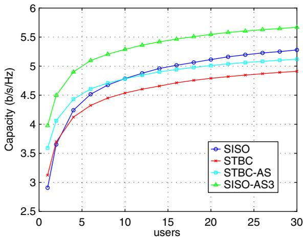
Fig. 3. Channel capacity vs. the number of active users for the different transmission schemes in an unlimited feedback scenario ( $\bar{\gamma} = 10$  dB).
