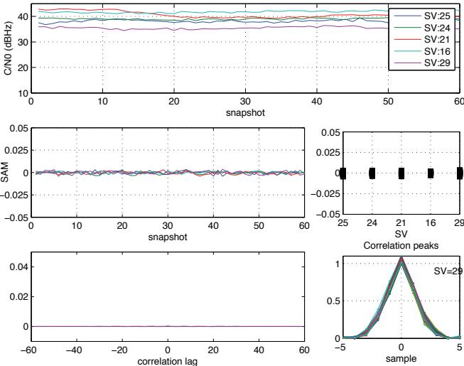
Fig. 5. (Top)  $C/N_0$  for satellites at position "p1". (Center) SAM. (Bottom Left) Correlation of SAM samples. (Bottom Right) Correlation peaks for the satellite with worst  $C/N_0$  value.
