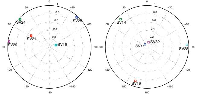
Fig. 4. (Left) Polar plot of visible satellites at "p1" in Fig. 2 on Jan 17, 2009, 09:01:46 GPS time. (Right) Polar plot of visible satellites at the canyon measurement position in Fig. 3 on Dec 22, 2008, 16:21:07 GPS time.
