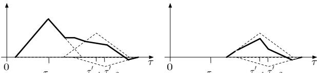
Fig. 1. Correlation peak when multipath is present. (Left) Scenario S1, line-of-sight is present. (Right) Scenario S2, line-of-sight is absent.
