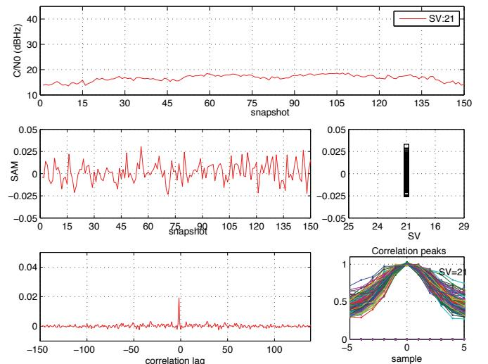
Fig. 10. (Top) Estimated C/N<sub>0</sub> values for visible satellites at position "p3". (Center) SAM. (Bottom Left) Correlation of SAM samples. (Bottom Right) Correlation peaks for SV21.
