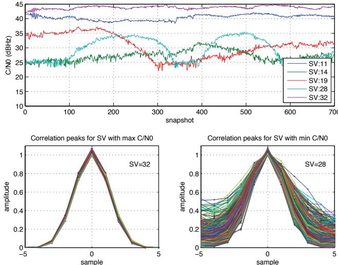
Fig. 8. (Top) Estimated C/N<sub>0</sub> values for the visible satellites at the canyon scenario. (Bottom) Correlation peaks for the satellites with maximum (left) and minimum (right) C/N<sub>0</sub> values at that scenario.
