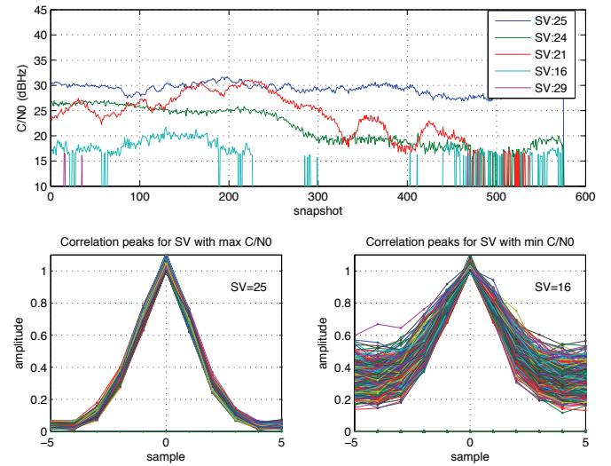
Fig. 6. (Top) Estimated  $C/N_0$  values for the visible satellites at position "p2". (Bottom) Correlation peaks for the satellites with maximum (left) and minimum (right)  $C/N_0$  values at that position.
