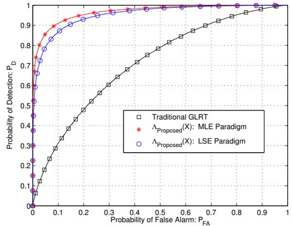
**Fig. 2.** Receiver Operating Characteristic (ROC) Curve:  $N = 40$ ,  $K = 36$ ,  $\sigma_s^2 = 2$ ,  $a_c = 0.3$ ,  $\beta = 2$
