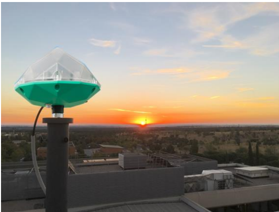
Figure 4 – Receiver GNSS two-antenna array
