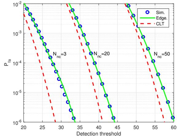
**Fig. 3.**  $P_{fa}$  vs. detection threshold with  $N_{nc} = 3, 20$  and  $50$  for the E.4 and CLT approximations and the optimal non-coherent detector obtained from simulations.
