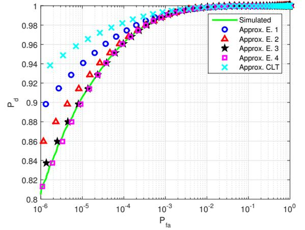
**Fig. 1.** ROC curve approximations for the performance of the optimal detector using the Edgeworth series and the CLT approximation for parameters:  $A = 1.7$ ,  $\sigma = 1$ , and  $N_{nc} = 10$ .
