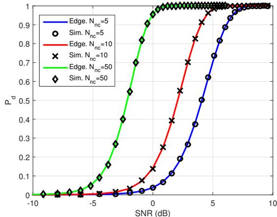
**Fig. 2.**  $P_d$  vs. SNR with  $N_{nc} = 5, 10, 50$  and  $P_{fa} = 1e-4$  for the E.4 approximation and the optimal non-coherent detector obtained from simulations.
