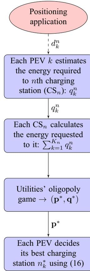
Figure 2. Oligopolistic game-theoretic framework for charging station selection: main steps
