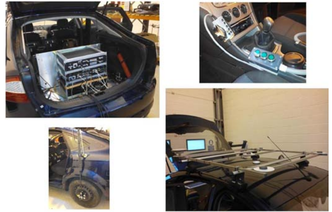
Figure 4- Vehicular DASU Assembly
