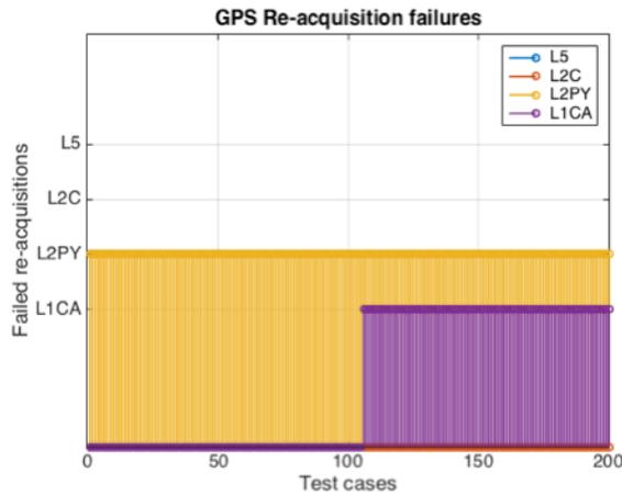
Figure 5: GPS signals re-acquisition test at  $C/N_0 = 30 \text{ dB-Hz}$ .
