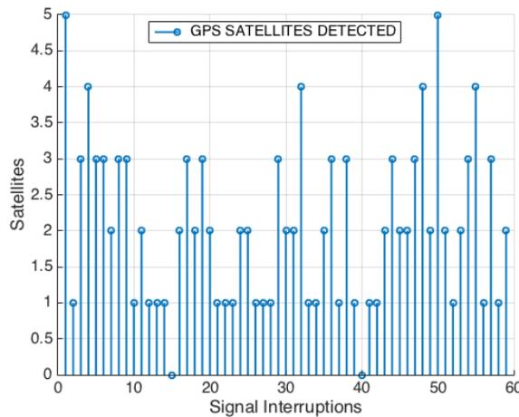
Figure 7. Satellite detection after losses of lock for low-mid latitude scintillation (C/N0 = 30dB-Hz).
