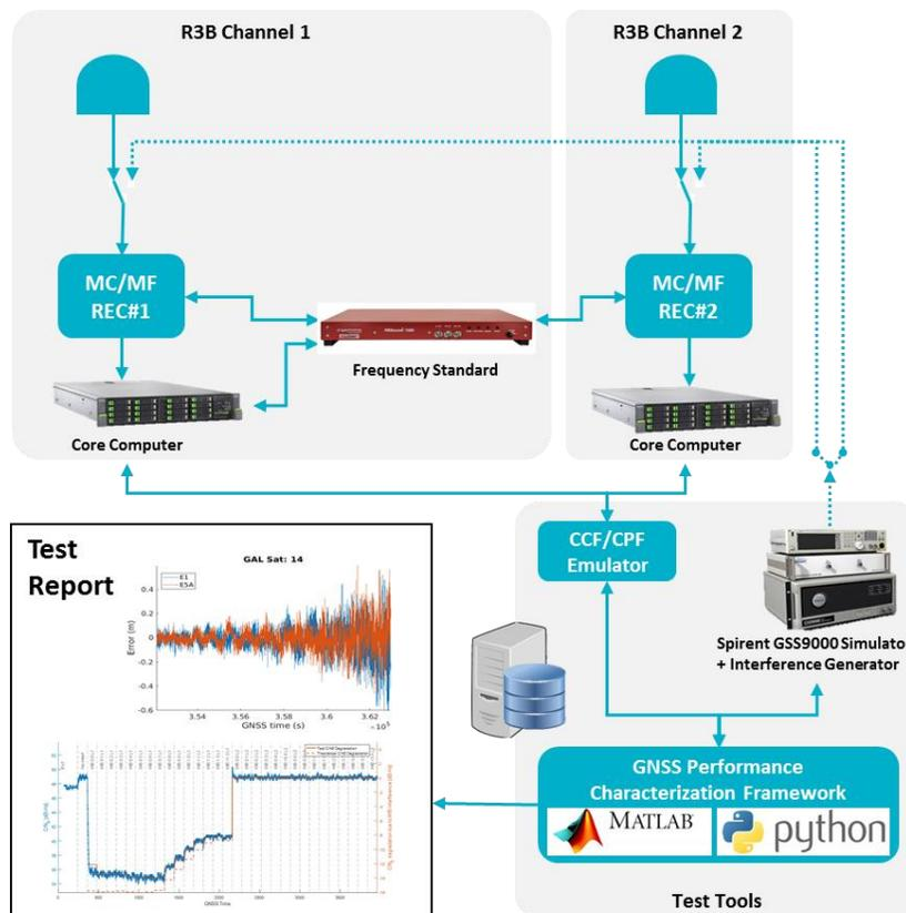
Figure 3. Advanced GNSS Reference Station for EGNOS v3 prototype with Characterization Framework
