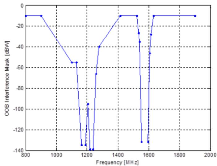
Figure 4: HYP-080 out-of band CW interference mask for all baseline signals
