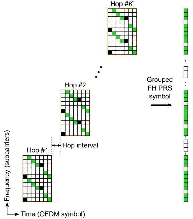
Fig. 2. Allocation scheme of the FH PRS for NB-IoT positioning.
