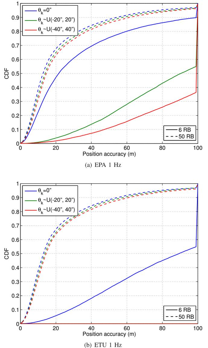
Fig. 7. Position accuracy with FH PRS covering a 6-RB and 50-RB signal bandwidth for different phase offset distributions and a group delay of  $-10$  ns.
