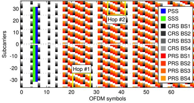
Fig. 3. Two hops over an in-band PRS transmission of 6 RB.
