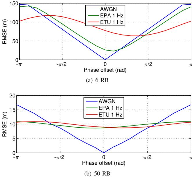
Fig. 6. Impact of the phase offset on the RMSE of the TDE with two hops over 6 and 50 RB for  $C/N_0 = 90$  dB-Hz without group delay, i.e.,  $\Delta_k = 0$ , by using 1000 Monte-carlo simulations.
