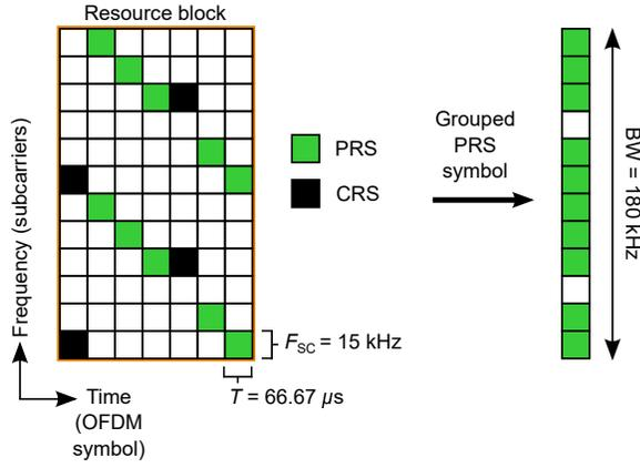
Fig. 1. Allocation pattern of the CRS and PRS within one RB.
