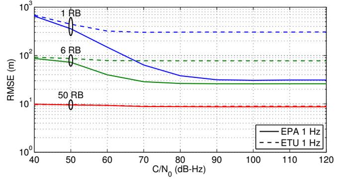
Fig. 4. RMSE of a threshold-based estimator for narrowband PRS of one RB and the FH PRS covering 6 RB and 50 RB, by using 1000 Monte-carlo simulations.
