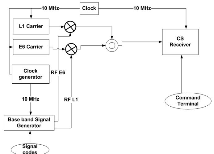
Figure 11 - Encrypted sample streaming setup
