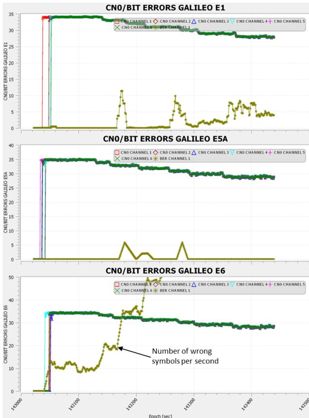
Figure 8 –  $C/N_0$  vs. wrong symbols per second (estimated by Viterbi decoder) in Galileo E1, E5a, E6-B
