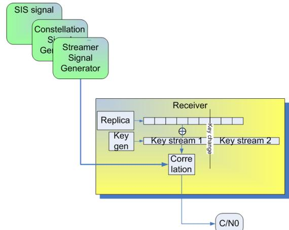
Figure 12 - Encrypted key change scheme
