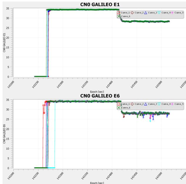
**Figure 7 - Acquisition and tracking behavior on Galileo E1/E6 for 6 satellites**
