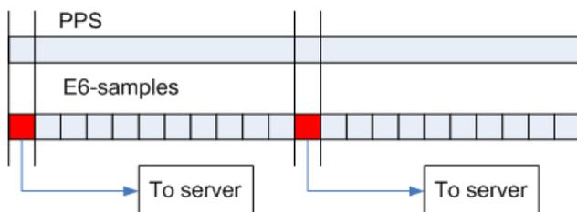
**Figure 6 - PPS steering setup of remote processing scheme**
