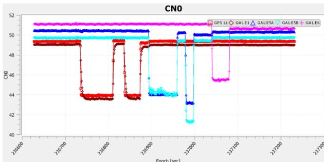
Figure 10 - Notch filter test result
