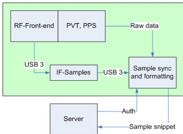
**Figure 5 – CS receiver architecture for Remote Processing Authentication**
