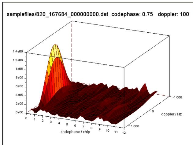
Figure 14 - Spreading code correlation with samples
