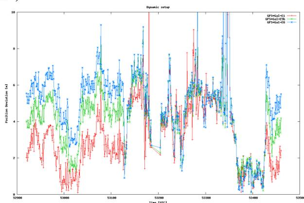
**Figure 18 - Position deviation in dynamic setup (red: GPS+Gal, E1; green: GPS+Gal, E5b; blue: GPS+Gal, E6)**
