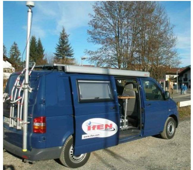
Figure 15 - Testing van for CS Receiver SIS testing
