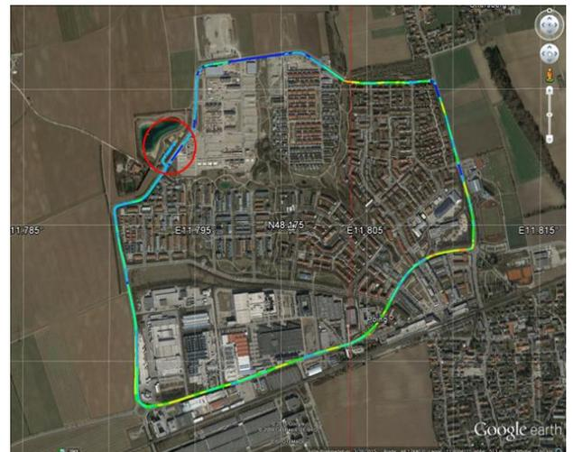
Figure 16 - Test trajectory for CS Receiver SIS testing
